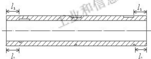
Figure 1 Testing sample tube with artificial notches
